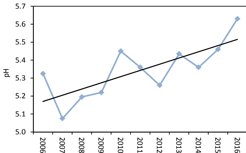
Above: Four Mile Branch at Lighthouse Drive showed an increase in stream pH during the 11-year study of water-quality trends. Graphic/John Bunnell
